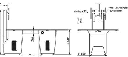
Designed primarily for collaboration, the **T628T** table brings a clean look to today's high-tech group environment. It features 42" bar height tabletop, two large base compartments designed to house racks or PC's; islands are designed to conceal inputs/outputs and power supplies.
